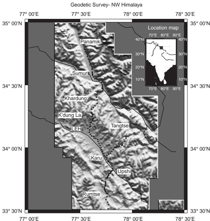
**Fig. 1.** Surface relief map of the Ladak region showing the GPS, levelling and gravity stations along the Rumtse–Panamik profile
