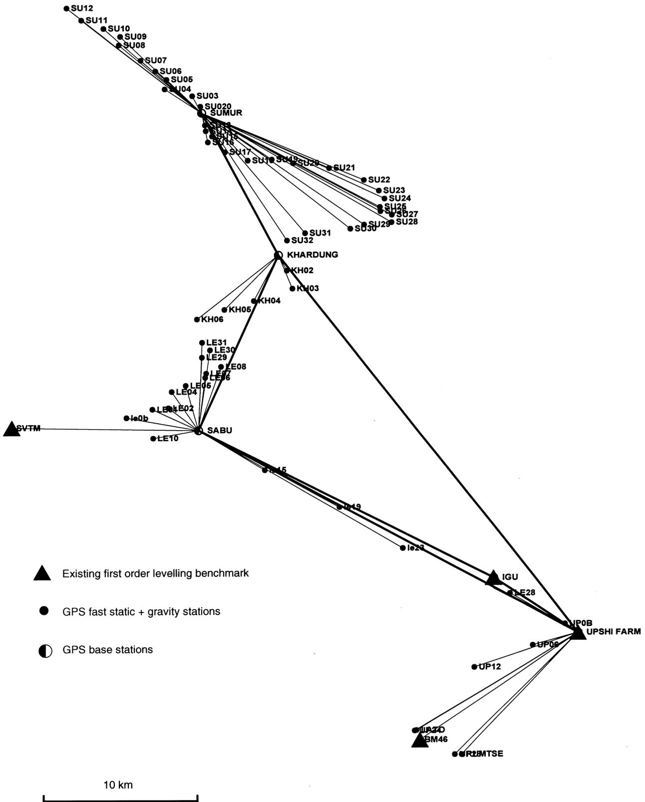
Fig. 2. Fast-static GPS network in Ladak. New levelling bench-marks are tied with existing first-order bench-marks. Leh (SABU) GPS base station is tied to Lhasa and Kitab IGS stations
