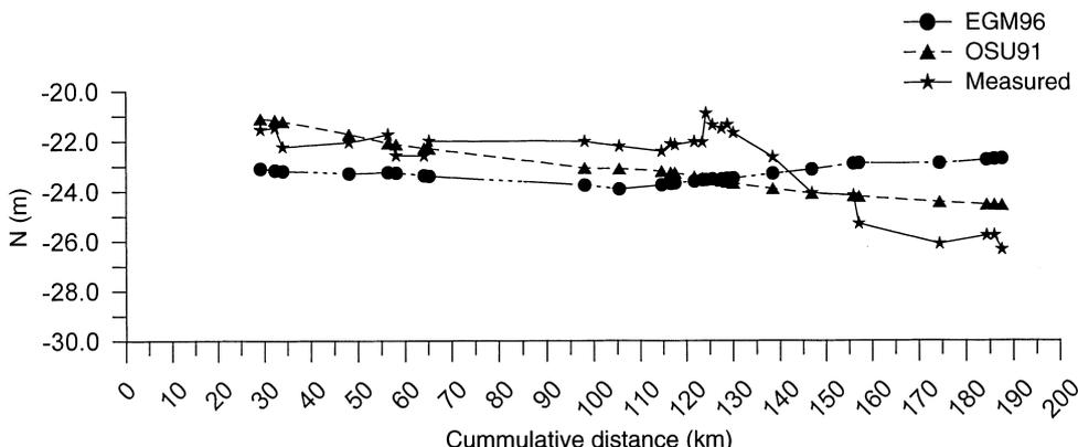
Fig. 3. A comparison of measured geoid undulation with EGM96- and OSU91-derived geoid models along Rumtse–Panamik section. OSU91 has a downward trend in the northern part in agreement with the measured geoid. In contrast, EGM96 model shows an upward trend in the northern part
