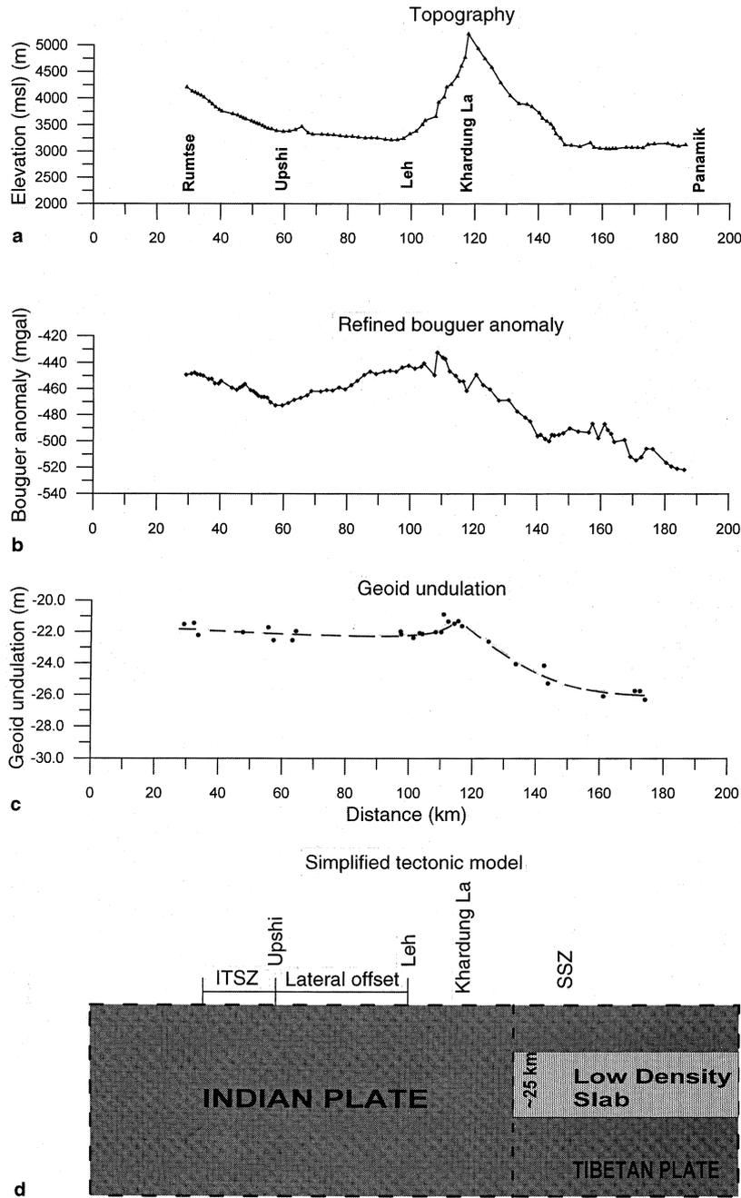
**Fig. 4a–d.** **a** Topography, **b** Bouguer gravity and **c** Geoid undulation anomalies along the Rumtse–Panamik profile. **d** Model of a 20–25-km-thick low-velocity layer within the Tibetan plateau. The actual plate boundary may be located north of Khardung La peak, beneath a granitic batholith, rather than at the Indus Tsangpo Suture Zone (ITSZ)
