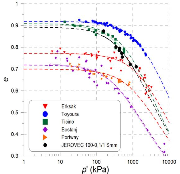
**Figure 6-3** The critical state line of Jerovec sand in comparison with the critical state lines of some other well known sands
