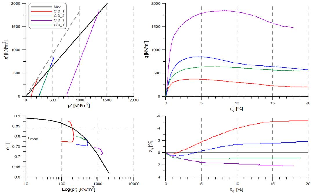
**Figure 6-1** The results of CID tests on Jerovec sand
