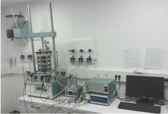
Figure 4-1 Triaxial apparatus at the Geotehnicki studio Ltd
