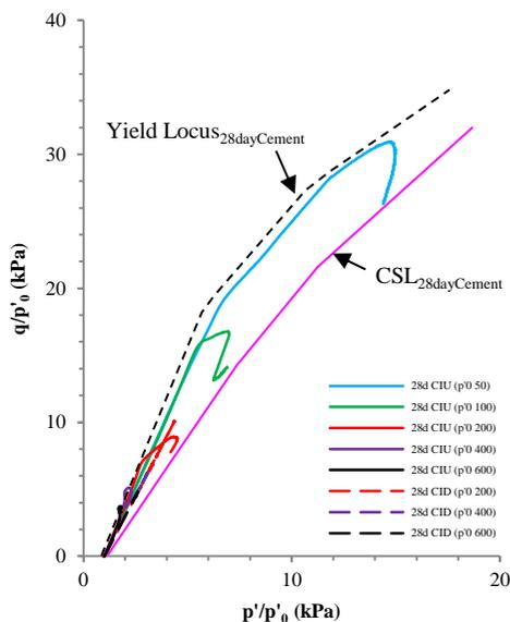
**Figure 5.**  $p'_{0}$  normalised effective Cambridge stress paths, CSL's and yield locus for 28d 7.5% GGBS-NaOH alluvium.
