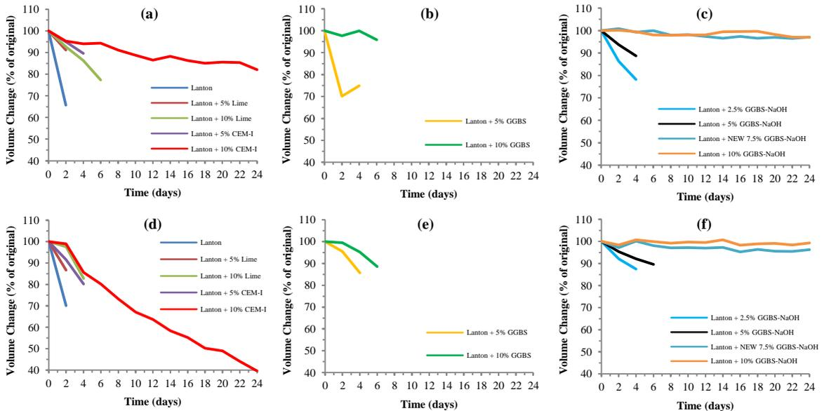
Figure 2. Volumetric changes experienced by samples during: (a-c) wetting-drying and (d-f) freezing-thawing testing.
