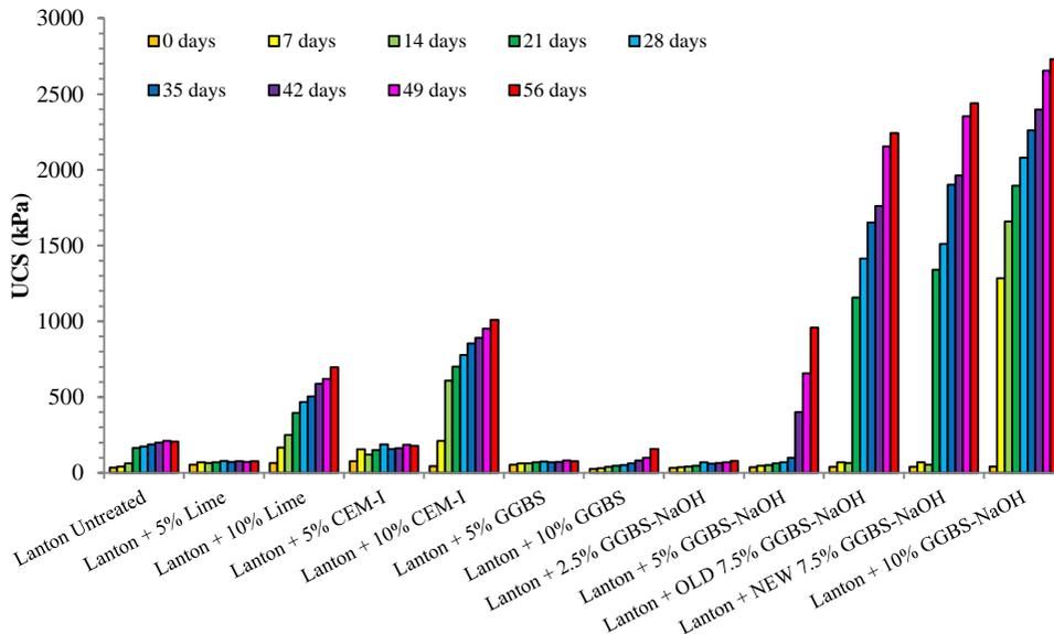
**Figure 1.** Unconfined compressive strength development for all binder mixtures and dosages used to stabilise Lanton alluvium.
