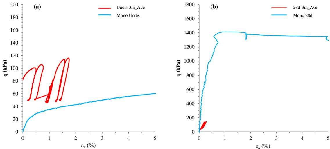
**Figure 6.** Cyclic (red) and respective monotonic (blue) deviatoric strengths at  $p'_0 = 60\text{kPa}$  for: (a) Undis and (b) 28d samples.
