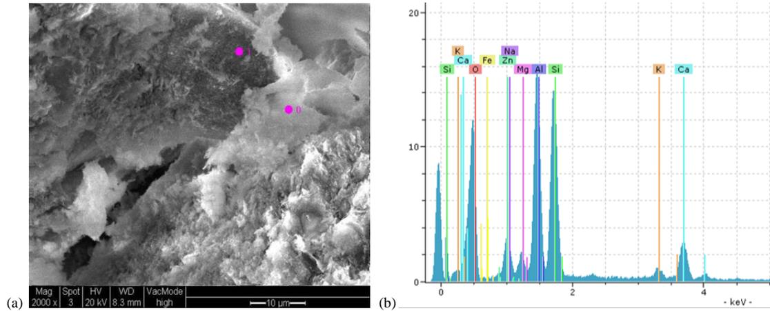
**Figure 3.** (a) SEM micrograph showing cement development within GGBS-NaOH stabilised alluvium after 56 days curing; (b) EDX spectra for point “0” on Figure 3a.
