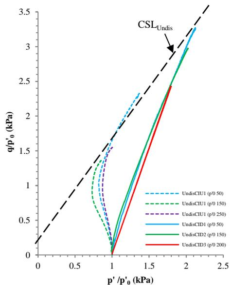
**Figure 4.**  $p'_0$  normalised effective Cambridge stress paths, CSL’s and yield loci for undisturbed alluvium.
