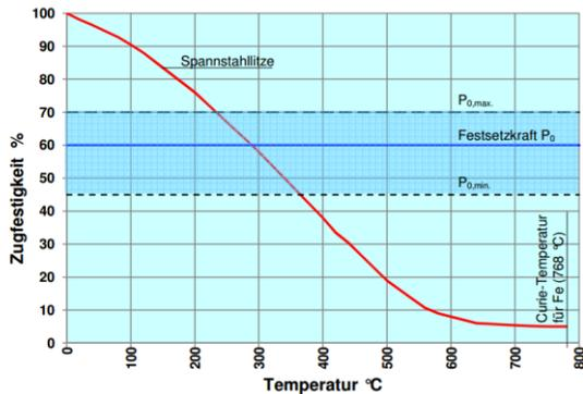
**Figure 9:** Evolution of strand strength (% of nominal strength) with temperature (source: Stahlton AG)
