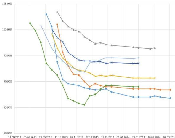
**Figure 7:** Anchor-Jet® load evolution with time
