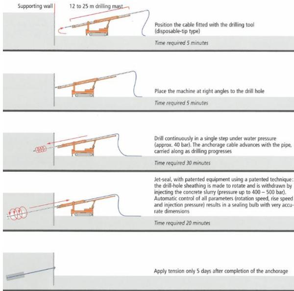
**Figure 2:** construction sequence of an Anchor-Jet® anchor (image: Forasol SA)
