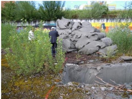
**Figure 1:** trial pit spoil heap demonstrates soil cohesion and softness
