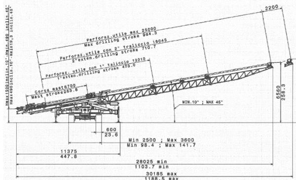
**Figure 3:** rig dimensions (image: Forasol SA)
