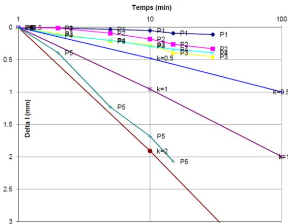
**Figure 5:** Pull-out test n°2 (bond length 5 m), P1 = 200 kN, increment 100 kN,  $P_{creep} = 600$  kN
