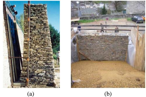
**Figure 2.** Experimental tests of DSRWs, loaded with: (a) hydrostatic force (Villemus et al. 2007); (b) backfill (Colas et al. 2010).
