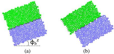
**Figure 3.** Kinematic of sliding failure during a tilt block test simulation with  $\phi_b^l=30^\circ$ : (a)  $\phi_b^g=20^\circ$ ; (b)  $\phi_b^g=31^\circ$ .
