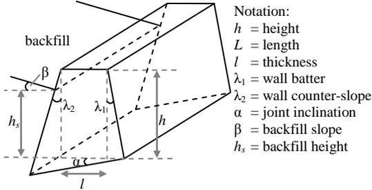
**Figure 1.** Geometry of a dry-stone retaining wall.
