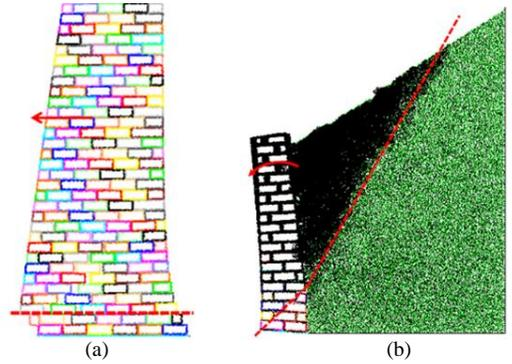
**Figure 8.** Failure modes of the DSRWs model: (a) sliding failure for case A; (b) toppling failure for case A and B.
