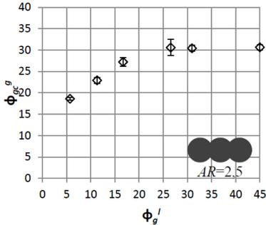
**Figure 4.** Backfill critical friction angle; influence of the local grain friction angle for an aspect ratio  $AR$  of 2.5.
