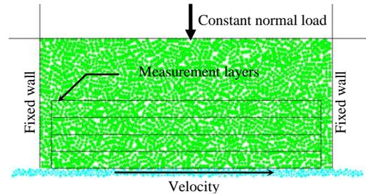
**Figure 6.** Simulation of an interface CNL test.
