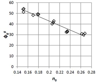
**Figure 5.** Backfill internal friction angle  $\phi_g^s$  according to the sample initial porosity  $n_0$  ( $AR=2.5$  and  $\phi_g^l=45^\circ$ ).
