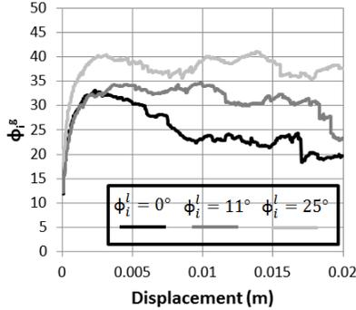
**Figure 7.** Evolution of the global interface friction angle according to the grain-block local friction angle.
