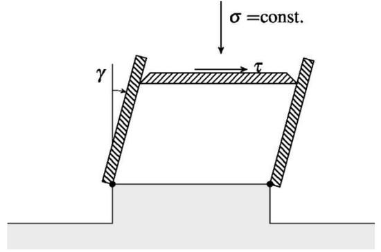
**Figure 2.** Schematic sketch of a Simple Shear test apparatus (c.f. Vermeer & de Borst 1984)
