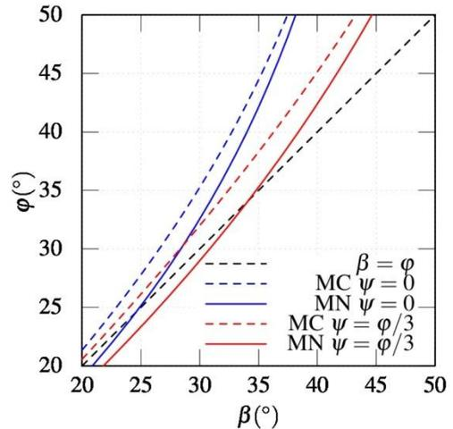
**Figure 9.** Maximum slope inclinations  $\beta$  for different dilatancy angles  $\psi$  and different friction angles  $\varphi$  with Mohr-Coulomb criterion (MC) and the Matsuoka-Nakai criterion (MN).
