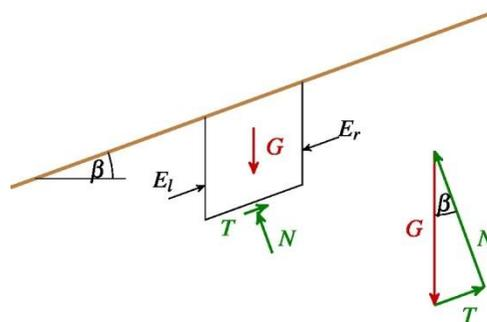
**Figure 1.** Element of the infinite slope with acting forces and vector sum of forces.
