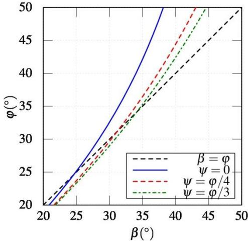
**Figure 8.** Maximum slope inclinations  $\beta$  for different dilatancy angles  $\psi$  and different friction angles  $\varphi$  with the Matusoka-Nakai criterion.
