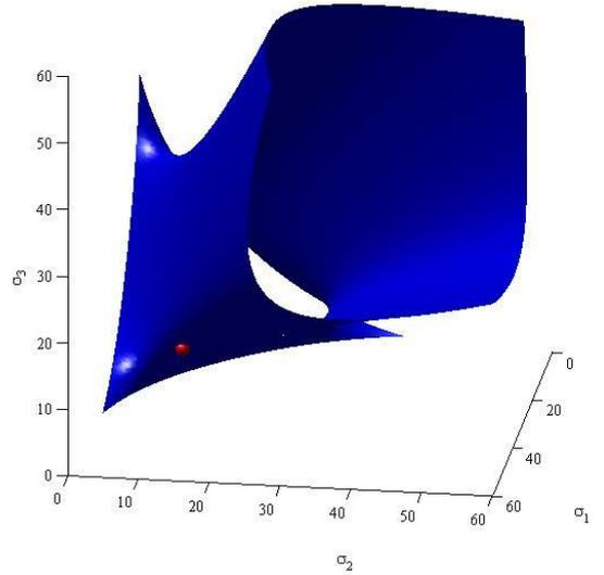
**Figure 6.** Matsuoka-Nakai plastic potential for  $\psi \neq \varphi$  and a given stress state on the Matsuoka-Nakai yield surface (red point;  $\varphi = 30^\circ$ ,  $\psi = 0$ ,  $g(\sigma) = 5453$ ) (c. f. Schranz 2014)
