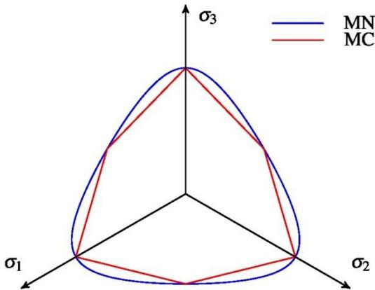
**Figure 5.** Intersection of Matsuoka-Nakai (MN) and Mohr-Coulomb (MC) criterion with a deviatoric plane for the same friction angle  $\varphi = 30^\circ$ .
