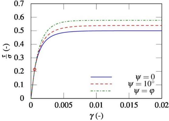
**Figure 3.** Shear stress as function of shear strain in a drained simple shear for different dilatancy angles (Material parameters:  $E = 20 \text{ MPa}$ ,  $\nu = 0.3$ ,  $\phi = 30^\circ$ ).
