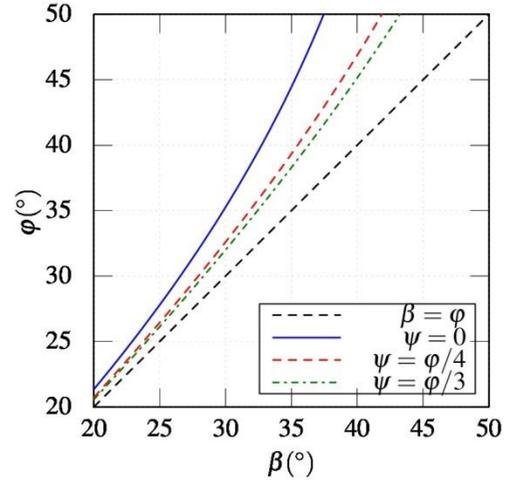
**Figure 4.** Maximum slope inclinations  $\beta$  for different dilatancy angles  $\psi$  and different friction angles  $\phi$ .
