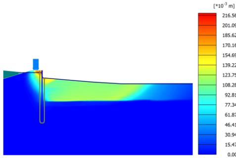
**Figure 7.** Soil displacements  $|u|$  [m] at full loading with design values and at safety factor corresponding to construction strength.
