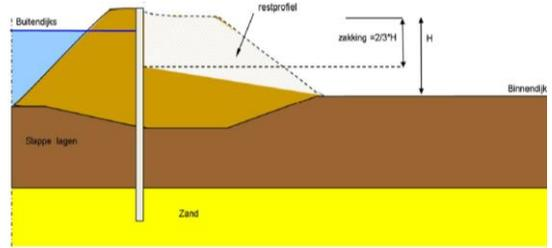
**Figure 2.** Residual profile for the inward stability.
