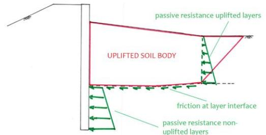
**Figure 6.** Schematic representation of the passive resistance.
