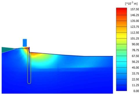
**Figure 3.** Soil displacements  $|u|$  [m] at full loading with design values and before strength reduction.
