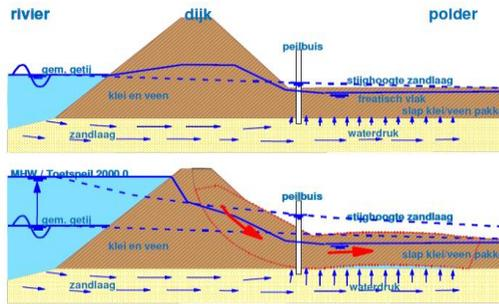
Figure 1. Illustration of the uplift phenomenon.
