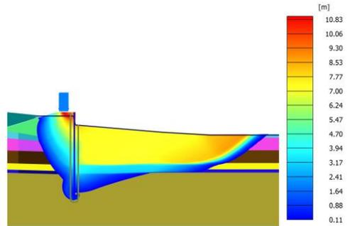
**Figure 5.** Soil displacements  $|u|$  [m] at full loading with design values and at end of strength reduction.
