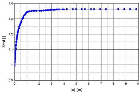
**Figure 4.** Safety factor vs. displacement of wall top during strength reduction.
