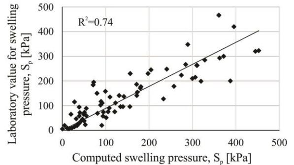
**Figure 4.** The correlation between the calculated values of the swelling pressure using the proposed equation and the values resulted from laboratory testing
