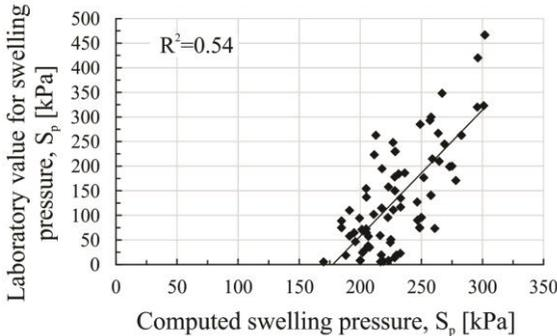
**Figure 6.** The correlation between the calculated values of the swelling pressure using the Sabtan's equation and the values resulted from laboratory testing
