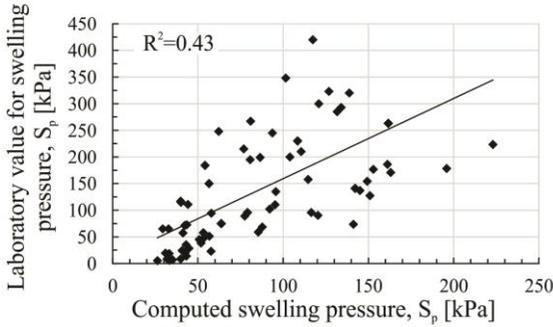
**Figure 5.** The correlation between the calculated values of the swelling pressure using Nayac's equation, and the values resulted from laboratory testing
