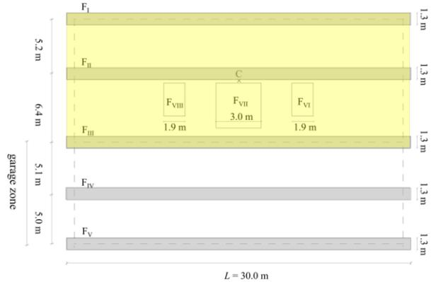
Figure 2. Plan view of the building's foundation system.
