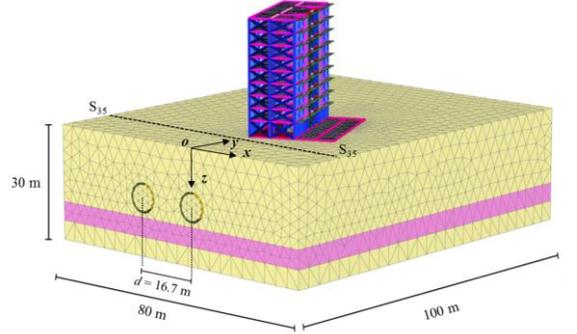
**Figure 4.** Finite element model and sketch of the mesh
