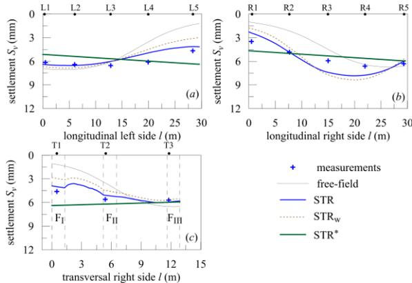
**Figure 9.** Comparison between measured and computed settlements with different structural models.
