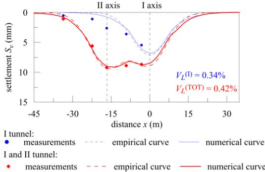
**Figure 6.** Comparison of computed profiles, Gaussian curves ( $K = 0.45$ ) and measured settlements.
