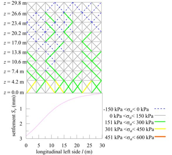
**Figure 8.** Axial stresses acting within the cross-bracings of the longitudinal left façade of the building.
