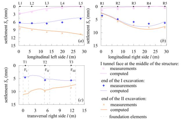
**Figure 7.** Comparison between measured and computed settlements along the building's façades during tunnelling.
