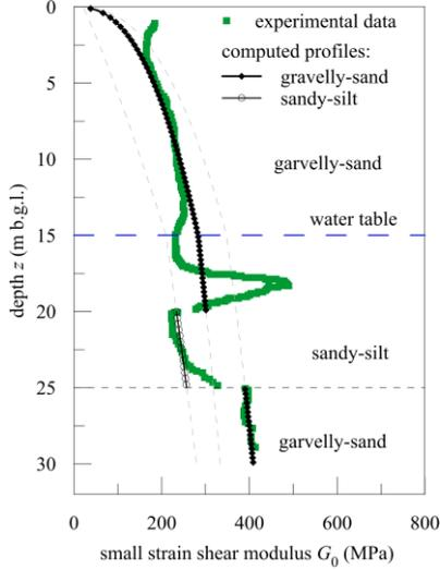
**Figure 3.** Experimental and computed  $G_0$ - $z$  profiles (the soil stratigraphy and the position of the water table are also shown).
