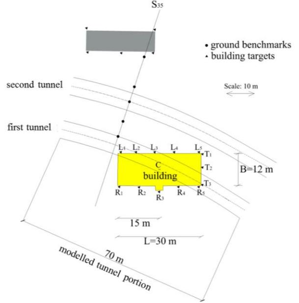
Figure 1. Detail of the examined portion of the route.
