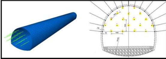
**Figure 2.** Layout of rock bolts
