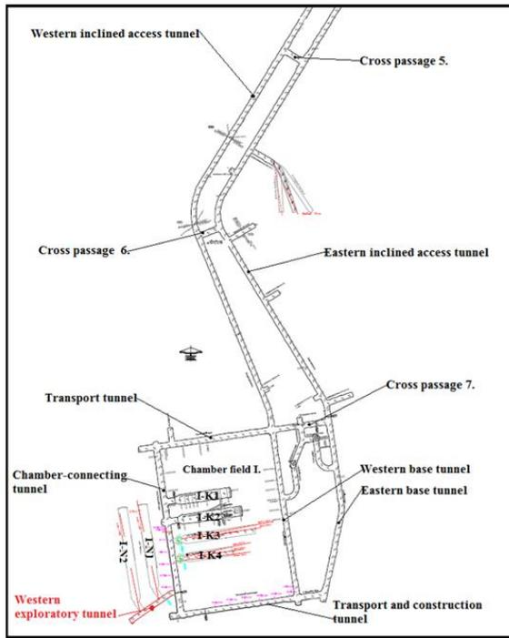
**Figure 1.** General layout of the repository (Kovacs et al. 2012)
