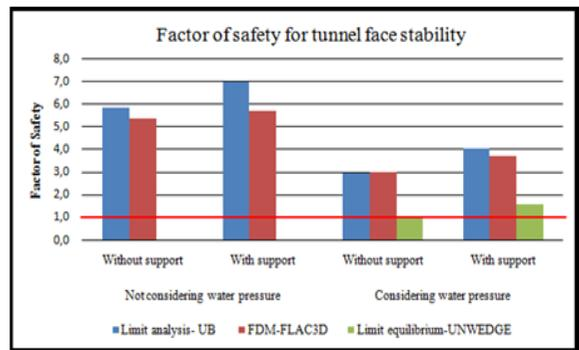
**Figure 3.** Factor of safety values (under 8.0) for tunnel face stability
