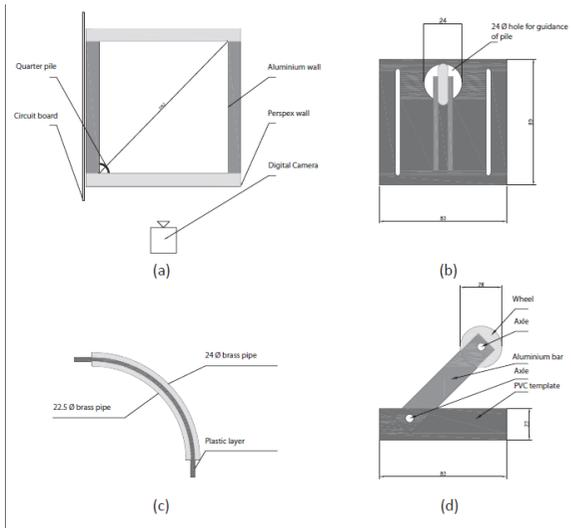
**Figure 1.** Pile and mechanical template; (a) top view of the strongbox, (b) top view of template, (c) top view pile, (d) side view template
