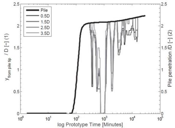
**Figure 4.** Development of neutral plane through time relatively to the pile base and the pile base displacement calculated from average incremental displacements of a 0.5D wide slice located at several distances in-between 0.5D – 3.5D
