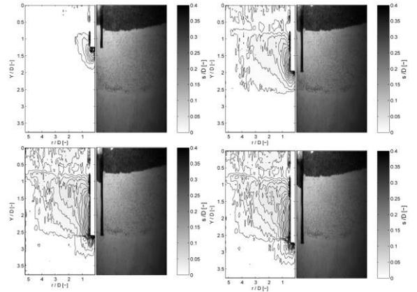
**Figure 2.** Contour plots of the total displacements in the soil at 4 penetration depths (1.25, 2.0, 2.6 & 2.75  $y/D$  [-]) during and immediate after installation
