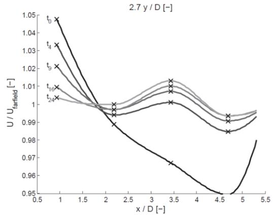
**Figure 3.** Dissipation of pore pressures near pile base after installation (subscript of  $t$  denotes prototype time in days) at 2.7  $y/D$
