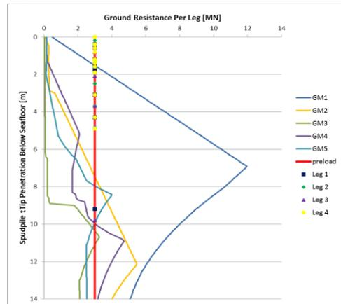
**Figure 6.** Spud pile penetration curve and registered pile penetration
