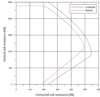
**Figure 7.** V-H interaction diagram, safety factor 1.1 on the foundation capacity and 1.25 in the sliding resistance.
