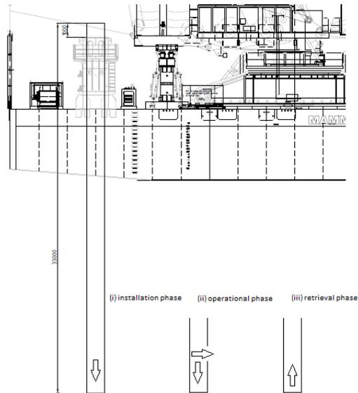
**Figure 4.** load cases (i) installation phase, (ii) operational phase and (iii) retrieval phase.
