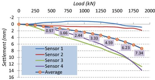
**Figure 4.** Load-settlement diagrams for sensors
