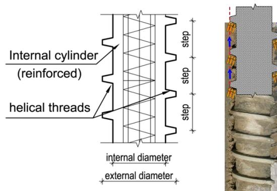
Figure 1. Screwsol pile
