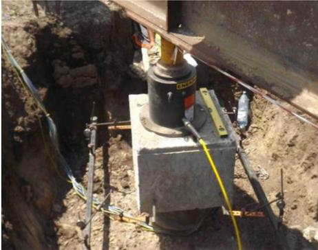
**Figure 5.** Pile head during load test.
