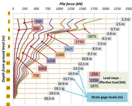
Figure 6. Pile forces for load steps
