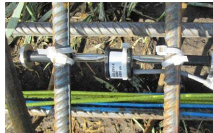
Figure 3. Strain gage installed on cage
