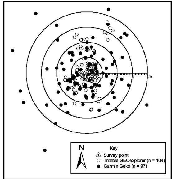
Fig. 3. Accuracy plots for the Garmin Geko and Trimble GeoXT: (a) plan view of recorded GPS positions relative to a known point collected over a fifty day period, (b) histogram showing horizontal errors in metres of GeoXT and Geko GPS positions and (c) probability vs. distance plot for GeoXT and Geko GPS positions.
