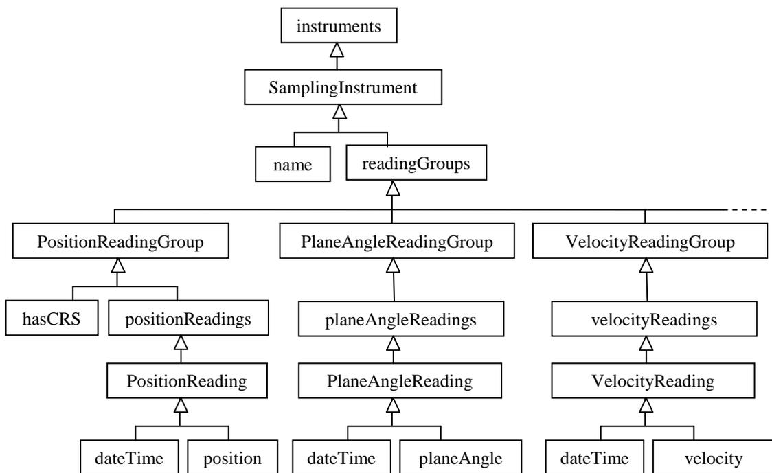
Fig. 5. Proposal for representing instruments within DIGGS (after Bray, 2007)
