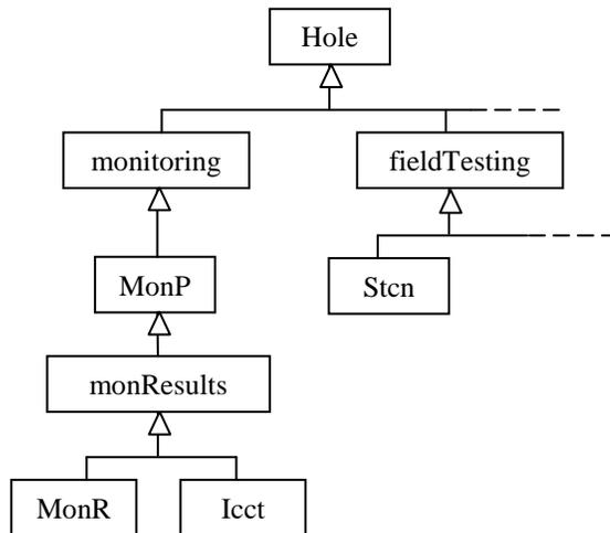
**Fig. 2. AGSML representation of monitoring data (after AGS, 2005)**
